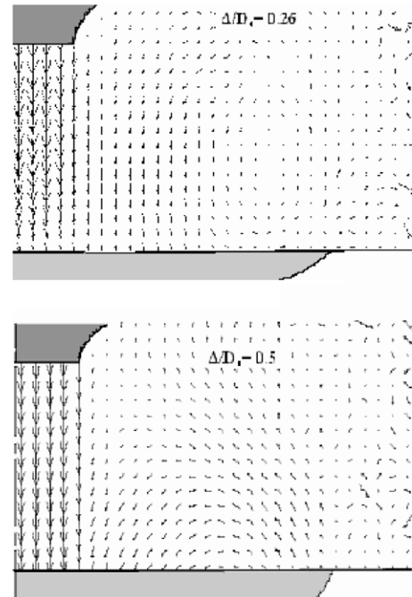
Fig. 3. The time-average flow pattern between the nozzle and the obstacle. Re = 1.2 \times 10^4 , S/d_0 = 2 .
